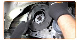
Tighten the fasteners of the lower timing cover. Use a drive socket #10. Use a torque wrench. Observe the recommended tightening torque.
