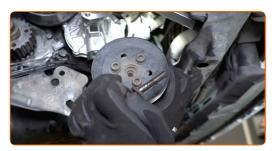
Tighten the fasteners of the hydraulic power steering pump. Use a drive socket #13. Use a drive socket #16. Use a torque wrench. Observe the recommended tightening torque.
