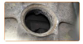
Turn the crankshaft gear. Use 12-point socket No.19. Use a ratchet wrench.
