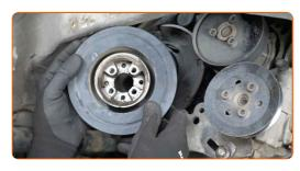
Clean the water pump pulley fastener. Use a wire brush. Use all-purpose cleaning spray.
