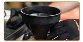
Pour coolant in the coolant reservoir.
