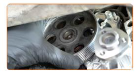
Tighten the vacuum pump pulley fastener. Use a universal pulley holder. Use a drive socket #19. Use a torque wrench. Observe the recommended tightening torque.
