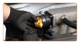
Release the air filter housing retainers. Remove the air filter housing.
