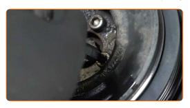
Remove the crankshaft pulleys.
