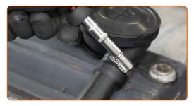
Remove the crankcase ventilation hose.
