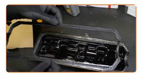
Install the engine valve cover.
