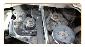
Remove the vacuum pump pulley.
