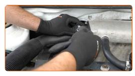
115 Remove the coolant reservoir cap.
