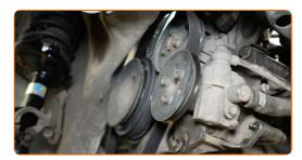
Clean the fastener of the crankshaft pulleys. Use a wire brush. Use WD-40 spray.
