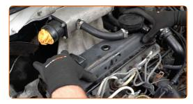
Tighten the engine valve cover fasteners. Use a drive socket #10. Use a torque wrench. Observe the recommended tightening torque.
