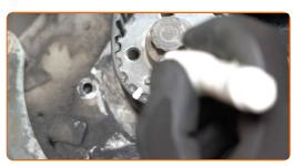
Loosen the fastener of the timing belt tensioner pulley. Use a drive socket #15. Use a ratchet wrench.
