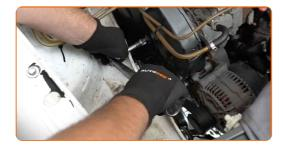
Tighten the alternator fasteners. Use a drive socket #13. Use a drive socket #16. Use a torque wrench. Observe the recommended tightening torque.
