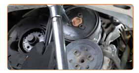
Install the crankshaft pulleys according to the factory marks.
