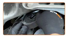
Unscrew the fasteners of the lower timing cover. Use a drive socket #10. Use a ratchet wrench.
