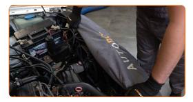
Unscrew the fasteners of the car battery terminals. Use a drive socket #10. Use a ratchet wrench.
