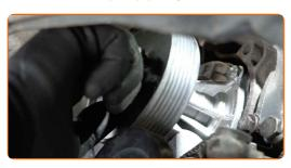
Tighten the water pump pulley fastener. Use HEX No.H6. Use a torque wrench. Observe the recommended tightening torque.
