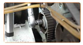
Remove the timing belt tensioner pulley.
