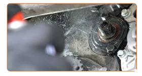
70 Install the vacuum pump pulley.
