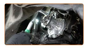
Treat the mounting seat of the vacuum pump pulley. Use all-purpose cleaning spray.
