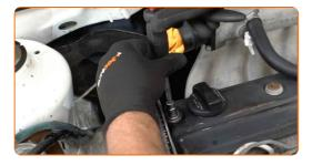
Remove the engine valve cover.
