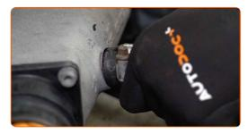
Fasten the clamp on the crankcase ventilation hose. Use a drive socket #7. Use a ratchet wrench.
