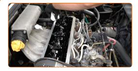
Treat the engine valve cover mounting seat. Use a sealant.
