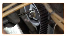
Remove the locking tool from the high pressure fuel pump pulley.
