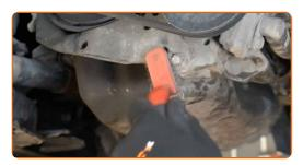
Unscrew the fasteners of the hydraulic power steering pump. Use a drive socket #13. Use a drive socket #16. Use a ratchet wrench.
