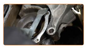
Treat the water pump mounting seat. Use a sealant.
