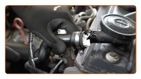
Unscrew the engine valve cover fasteners. Use a drive socket #10. Use a ratchet wrench.
