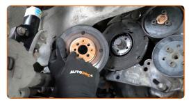
Tighten the fastener of the crankshaft pulleys. Use HEX No.H6. Use a torque wrench. Observe the recommended tightening torque.
