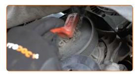
Unscrew the water pump pulley fastener. Use HEX No.H6. Use a ratchet wrench.
