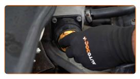
Reinstall the air distribution housing assembly.
