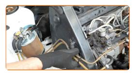
Tighten the fasteners of the upper timing cover. Use a drive socket #13. Use a torque wrench. Observe the recommended tightening torque.
