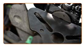
Remove the camshaft locking tool.
