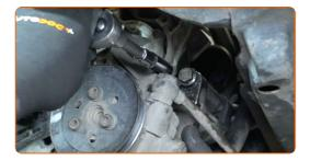
Remove the hydraulic power steering pump.
