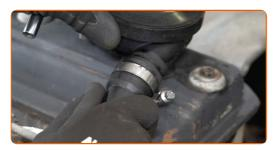
Cover the PCV valve hole with a microfibre cloth to prevent dirt and foreign objects from getting into the system.
