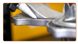
66 Install the water pump gasket.
