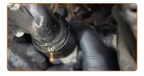
Drain the coolant from the engine.
