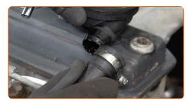
Detach the crankcase ventilation hose clamp. Use a drive socket #7. Use a ratchet wrench.
