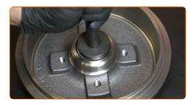
Treat the inner race and the wheel bearing. Use a multipurpose grease.
