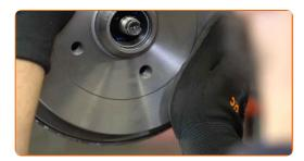
Apply special grease to the bearing assembly mounting seat. Use a multipurpose grease.
