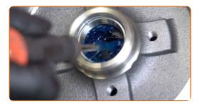
15 Install a new hub bearing and secure it.
