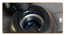
Clean the stub axle. Use all-purpose cleaning spray. Use WD-40 spray.
