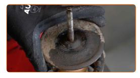
Release the coil spring.
