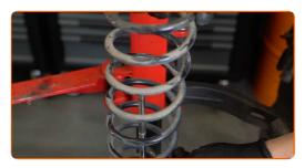
Install the spring on the shock absorber.
