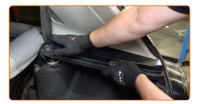
Screw the fasteners of the side plastic trim panel. Use a drive socket #10. Use a ratchet wrench.
