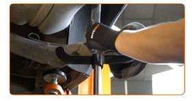
Unscrew the lower fastener of the shock absorber strut. Use a combination spanner #17. Use a drive socket #17. Use a tap wrench.
