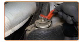
Loosen the upper fastener of the shock strut mount. Use a combination spanner #17. Use a shock absorber socket #DD5,2. Use a ratchet wrench.
