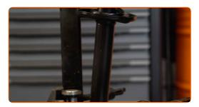
Treat the mounting seats of the shock strut. Use a wire brush. Use WD-40 spray.
