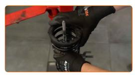
Install the dust boot and bump stop on the shock absorber.
