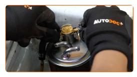
13 Install the fuel line retaining clip.
