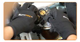
Screw the fastener attaching the fuel supply line to the fuel filter housing. Use a drive socket #7. Use a ratchet wrench.
