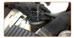
Screw in the fuel filter mounting bracket. Use a drive socket #13. Use a ratchet wrench.
