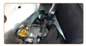
Loosen the fuel supply lines fastening to the fuel filter. Use a drive socket #7. Use a ratchet wrench.
