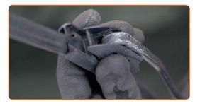
Remove the blade from the wiper arm.
