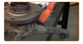
Install the brake disc cover.
