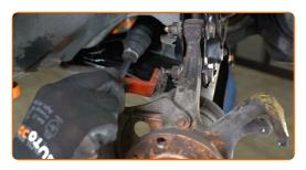
Unscrew the fasteners connecting the suspension strut to the steering knuckle. Use a combination spanner #18. Use a drive socket #18. Use a ratchet wrench.
