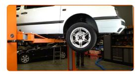
Tighten the drive shaft nut. Use a drive socket #30. Use a torque wrench. Tighten it to 230 Nm torque.
