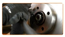
15 Remove the brake disc.
