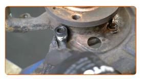
Remove the brake disc cover.
