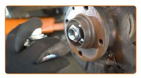
64 Install the brake disc.
