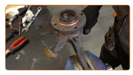
Clean the mounting seat of the brake disc cover. Use a wire brush. Use WD-40 spray.
