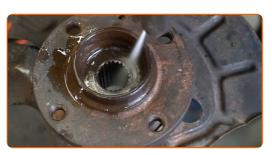
Release the vice and remove the steering knuckle assembled with the wheel hub.
