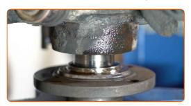
Place the steering knuckle assembled with the wheel hub in a vice.
