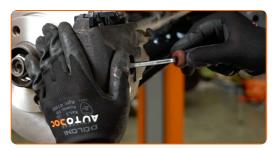
Remove the brake caliper.
