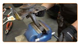
Treat the shock strut mounting seat on the steering knuckle. Use a wire brush. Use WD-40 spray.
