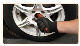
Loosen the fastener of the driveshaft. Use a drive socket #30. Use a tap wrench.
