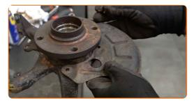
Screw in the fasteners of the brake disc cover. Use a combination spanner #10.
