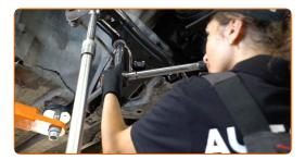
Tighten the fasteners connecting the ball joint to the control arm. Use a drive socket #13. Use a torque wrench. Tighten it to 35 nm torque.
