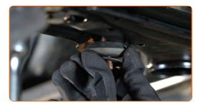
Install the rod fastening to the stabilizer and tighten it. Use a drive socket #13. Use a torque wrench. Tighten it to 25 Nm torque.
