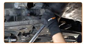
Unscrew the rear fastener connecting the control arm to the subframe. Use a drive socket #18. Use a tap wrench.
