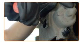
11 Remove the brake caliper.
