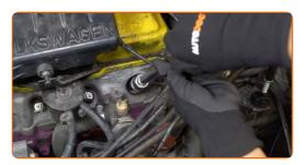
Screw new spark plugs and tighten them. Use the spark plug socket #21. Use a torque wrench. Tighten it to 25 nm torque.
