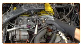
Unscrew the spark plugs. Use the spark plug socket #21. Use a ratchet wrench.
