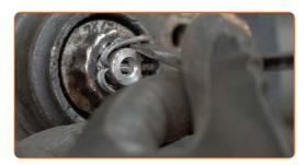
Unscrew the hub nut. Use a drive socket #30. Use a ratchet wrench.
