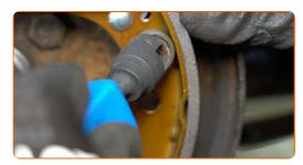
Install the lower return spring. Use a crowbar. Use a flat screwdriver.
