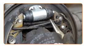
Remove the brake shoe hold-down cup. Use a brake shoe retaining spring compressor.
