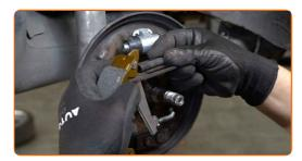
Install the brake shoes on the working brake cylinder on the bracket and on the brake-support plate bracket.
