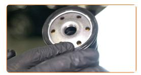
Screw the new filter into its place. Use the 74-15F socket. Use a torque wrench. Tighten it to 25 Nm torque.
