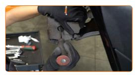
11 Remove the brake caliper.
