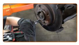
15 Remove the brake disc.
