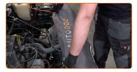
Unscrew the coolant reservoir cap.
