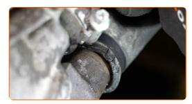
Drain the coolant from the engine.
