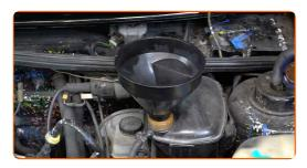
Pour coolant in the coolant reservoir.
