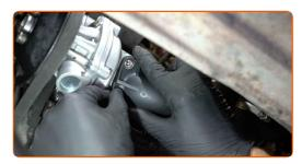
Tighten the thermostat housing fasteners. Use a drive socket #10. Use a torque wrench. Tighten it to 13 nm torque.
