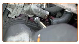
Remove the thermostat housing.
