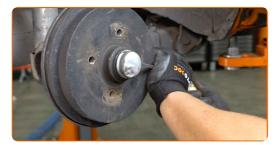
Remove the cotter pin securing the hub nut. Use a crowbar. Use a flat screwdriver.
