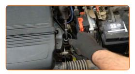
Release the air filter cover clips.
