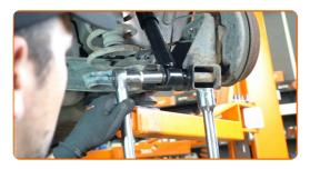
Tighten the top shock absorber fastening. Use a drive socket #15. Use a torque wrench. Tighten it to 70 Nm torque.
