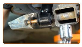
Screw in the lower fastener of the shock absorber. Use a drive socket #19. Use a ratchet wrench.
