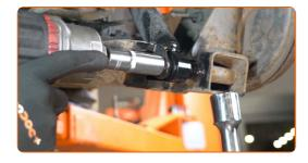
11 Remove the fastening bolt.
