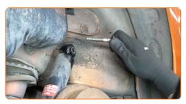
Unscrew the lower fastener of the shock absorber. Use a drive socket #19. Use a ratchet wrench.
