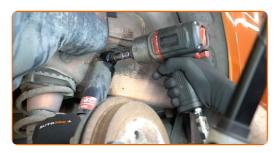
9 Remove the fastening bolt.
