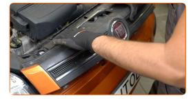
Use the masking tape to prevent plastic and painted parts of the car from being damaged.
