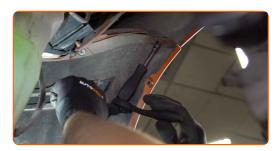
6 Unscrew the radiator grille fastener. Use a Phillips screwdriver.
