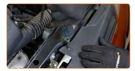
Screw in the lower fasteners of the bumper. Use a drive socket #8. Use Torx T30. Use a ratchet wrench.
