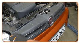
Screw in the fastener of the radiator grille. Use a Phillips screwdriver.
