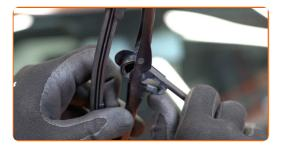
Remove the blade from the wiper arm.
