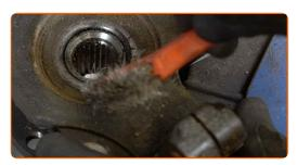
Remove the wheel hub from the steering knuckle. Use a bush and bearing driver set.
