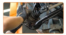
75 Tighten the brake caliper bracket. Use a drive socket #18. Use a torque wrench. Tighten it to 55 Nm torque.
