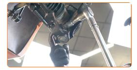
Tighten the lower fasteners connecting the shock strut to the steering knuckle. Use a combination spanner #15. Use a drive socket #17. Use a torque wrench. Tighten it to 75 Nm torque.
