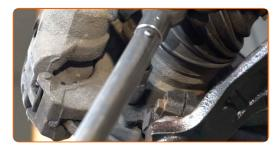
Treat the shock strut fasteners. Treat the fastener connecting the tie rod end to the steering knuckle. Treat the fasteners of the ball joint. Use copper grease.
