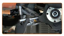
Clean the ABS sensor mounting seat. Use a wire brush. Use WD-40 spray.
