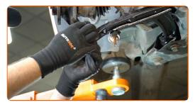
Screw the fastener connecting the ball joint to the steering knuckle. Use a combination spanner #13. Use a drive socket #16. Use a ratchet wrench.
