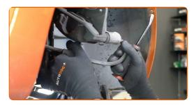
Unscrew the fastener connecting the ball joint to the steering knuckle. Use a combination spanner #13. Use a drive socket #16. Use a ratchet wrench.
