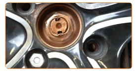
Tighten the wheel bolts using a criss-cross pattern. Use wheel impact socket #17. Use a torque wrench. Tighten it to 98 Nm torque.
