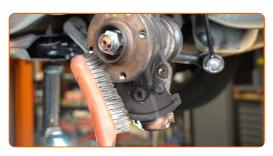
Treat the ABS sensor fastener. Use a multipurpose grease.
