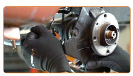
Screw on the fastening nut that connects the tie rod end to the steering knuckle. Use a drive socket #17. Use a ratchet wrench.
