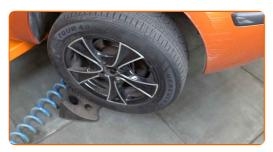
Unscrew the wheel bolts. Use wheel impact socket #17.
