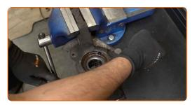
Remove the wheel hub bearing retaining ring. Use flat screwdrivers (2 pieces).
