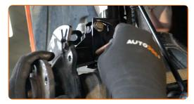
Screw in the fasteners connecting the suspension strut to the steering knuckle. Use a combination spanner #15. Use a drive socket #17. Use a ratchet wrench.
