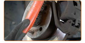
Unstake the fastener of the driveshaft. Use a flat metal-working chisel. Use a hammer.
