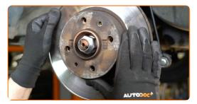
Tighten the brake disc fastening. Use a drive socket #12. Use a torque wrench. Tighten it to 9 Nm torque.
