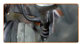
Connect the fastener of the ABS sensor cable to the shock absorber strut. Fasten the brake hose on the strut.
