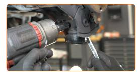
Remove the fastening bolt.
