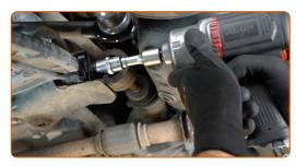
10 Remove the front fastener of the control arm.
