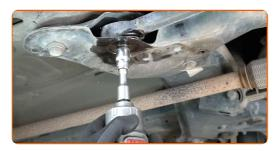
Remove the rear fastener of the control arm.
