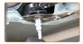
Screw the fastener connecting the ball joint to the steering knuckle. Use a combination spanner #13. Use a drive socket #16. Use a ratchet wrench.
