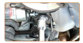
Tighten the ball joint fastener. Use a combination spanner #13. Use a drive socket #16. Use a torque wrench. Tighten it to 32 Nm torque.
