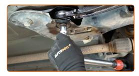
Remove the support from under the arm.
