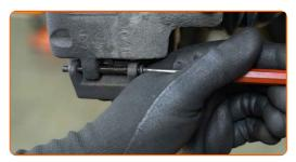
Install the lock pin retainer clip. Use round-nose pliers.
