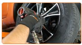
Lower the car and working in a cross order, tighten the wheel bolts. Use wheel impact socket #17. Use a torque wrench. Tighten it to 98 nm torque.
