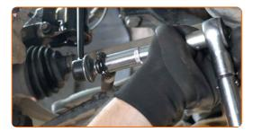
Tighten the fastener connecting the stabilizer link to the shock strut. Use a drive socket #17. Use a torque wrench. Tighten it to 23 Nm torque.
