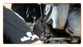
Tighten the fastener connecting the stabilizer link to the stabilizer bar. Use a drive socket #17. Use a torque wrench. Tighten it to 23 Nm torque.
