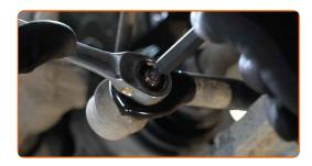
Unscrew the fastener connecting the stabilizer link to the shock strut. Use a drive socket #16. Use a ratchet wrench.
