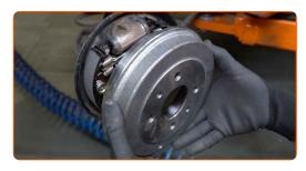
Move the parking brake shoes against the drum. Use a flat screwdriver.
