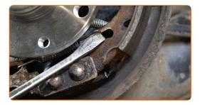
Remove the hold-down pins of the brake shoes. Use round-nose pliers.
