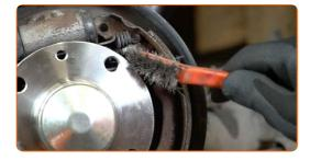
Remove the lower return spring of brake shoes. Use a crowbar.
