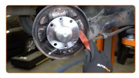
Install the upper retaining springs and adjustment mechanism on new brake shoes.
