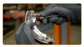
Clean the mounting seats of the brake shoes. Use a wire brush. Use all-purpose cleaning spray.
