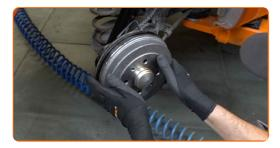
Screw in the brake drum fastener. Use a drive socket #12. Use a ratchet wrench.
