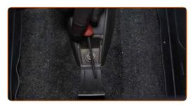
Unscrew the front fasteners of the lower centre console. Use a drive socket #10. Use a ratchet wrench.
