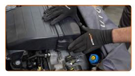
12 Remove the fender protection cover.
