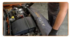
Release the air filter cover clips.
