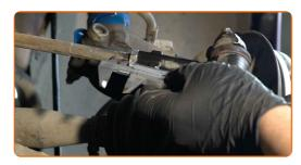
Loosen the lock nut securing the tie rod end to the tie rod. Use a combination spanner #22.
