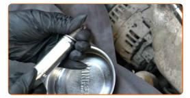
Apply a thin layer of special grease on the thread surface of new spark plugs. Use copper grease.
