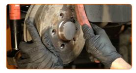
Treat the surface where the wheel rim contacts the brake drum. Use copper grease.
