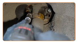
10 Remove the fastening bolt.
