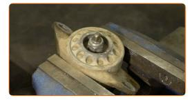
Clean the shock absorber rod fastener. Use a wire brush. Use WD-40 spray.
