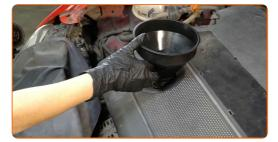
Pour oil into the engine through the filler. Required amount of oil: 3.2 l.
