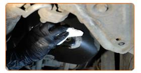
Screw in the new drainage plug and tighten it. Use a drive socket #19. Use a torque wrench. Tighten it to 27 Nm torque.
