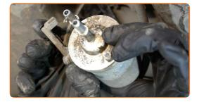
Clean the fasteners of the fuel supply lines. Use all-purpose cleaning spray.
