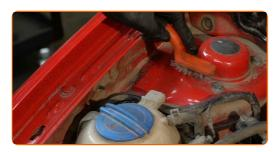
Loosen the upper fastener of the shock strut mount. Use a drive socket #13. Use a ratchet wrench.
