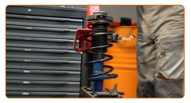
Remove the assembled shock strut.
