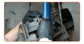
Install the brake hose retaining clip.
