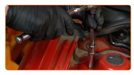
Remove the protective cap from the shock absorber strut mount.
