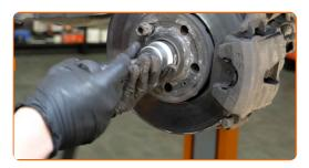
Tighten the drive shaft nut. Use a drive socket #36. Use a torque wrench. Tighten it to 50 Nm torque.+45°
