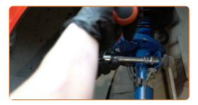
Treat the shock strut fasteners. Treat all joints of the arm. Use copper grease.
