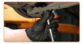
Disconnect the spherical joint from the arm.
