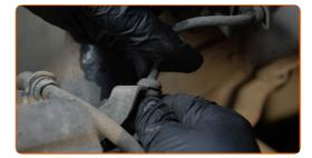
Clean the fasteners connecting the shock strut to the steering knuckle. Use a wire brush. Use WD-40 spray.
