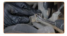
Disconnect the ABS sensor wiring.
