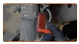
17 Remove the brake hose retaining clip.
