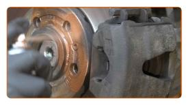
69 Clean the brake disk surface. Use a brake cleaner.
