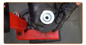
Tighten the shock strut piston rod nut. Use HEX No.H7. Use a drive socket #21. Use a torque wrench.
