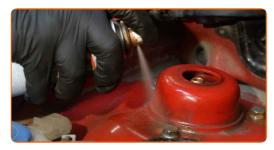
Install the protective cap onto the shock absorber strut mount.
