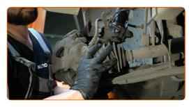
Prop up the steering knuckle. Use a hydraulic transmission jack.
