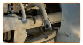
Replacement: anti roll bar links – Seat Ibiza 6L1. Tip from AUTODOC:
