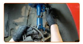
Tighten the fastener connecting the stabilizer link to the shock strut. Use a combination spanner #17. Use a drive socket #17. Use a torque wrench. Tighten it to 40 Nm torque.
