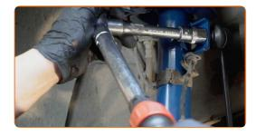
Tighten the fastener connecting the stabilizer link to the stabilizer bar. Use a combination spanner #17. Use a drive socket #17. Use a torque wrench. Tighten it to 40 Nm torque.
