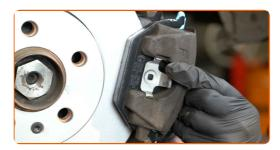
18 Install the dust boot caps of the brake caliper guide pins.
