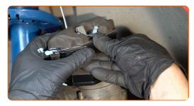
Install the brake caliper and fix it. Use HEX No.H7. Use a torque wrench. Tighten it to 28 Nm torque.
