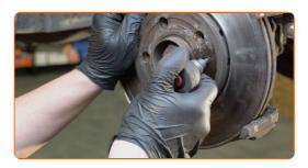
14 Remove the brake disc.
