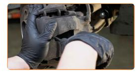
10 Remove the brake caliper.
