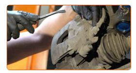
8 Unscrew the brake caliper fastening. Use HEX No.H7. Use a ratchet wrench.
