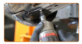
Disconnect the spherical joint from the arm.
