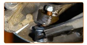
Screw the fasteners of the ball joint. Use a combination spanner #19.
