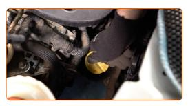
Run the engine for a few minutes. After the oil pressure warning light goes out, stop the engine.
