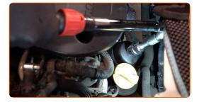
Install the protective case of the oil filter housing.
