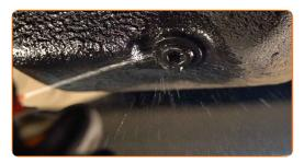
Unscrew the drain plug. Use HEX No.H14. Use a ratchet wrench.
