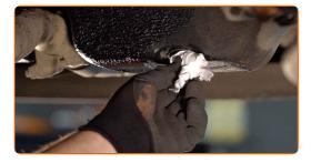
Screw in the new drainage plug and tighten it. Use HEX No.H14. Use a torque wrench. Tighten it to 22 Nm torque.
