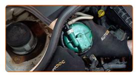
Clean the connector of the fuel pressure sensor. Use electronic spray.
