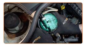
14 Attach the fuel pressure sensor connector.
