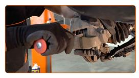
Remove the brake caliper.
