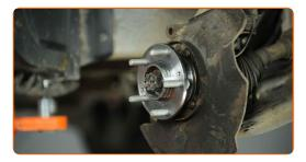
Tighten the wheel hub nut. Use a drive socket #32. Use a torque wrench. Tighten it to 195 Nm torque.
