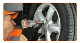
Lower the car and working in a cross order, tighten the wheel bolts. Use wheel impact socket #21. Use a torque wrench. Tighten it to 108 Nm torque.
