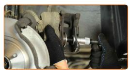
19 Install the brake caliper and fix it.
