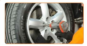
Lower the car and working in a cross order, tighten the wheel bolts. Use wheel impact socket #21. Use a torque wrench. Tighten it to 108 Nm torque.
