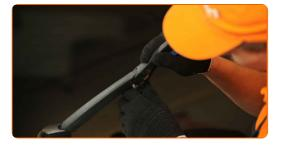
Remove the blade from the wiper arm. Use a flat screwdriver.
