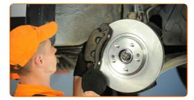
Tighten the brake caliper bracket. Use a combination spanner #17. Use a drive socket #17. Use a torque wrench. Tighten it to 85 Nm torque.
