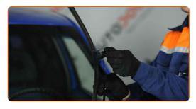
Remove the blade from the wiper arm.
