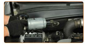
Screw in the water-in-fuel sensor.
