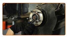
Unscrew the hub nut. Use a drive socket #32. Use a ratchet wrench.
