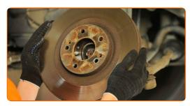
Clean the hub. Use a wire brush. Treat the contacting surface. Use high-temperature grease.
