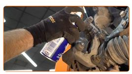
Unscrew the caliper bracket fastening. Use a drive socket #17. Use a ratchet wrench.
