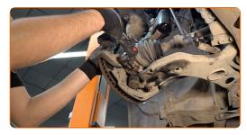
16 Remove the caliper bracket.
