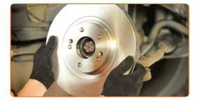
Tighten the brake disc fasteners. Use a Phillips screwdriver. Use a torque wrench. Tighten it to 6 Nm torque.
