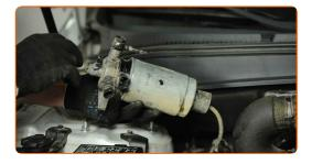
8 Unscrew the water-in-fuel sensor.
