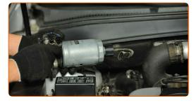
Screw in the water-in-fuel sensor.
