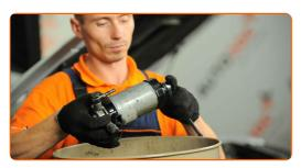
Remove the fuel filter fastening bracket. Remove the fuel filter.
