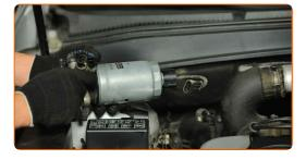
Screw in the water-in-fuel sensor.
