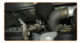
19 Attach the fuel pressure sensor connector.
