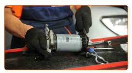
Install the new fuel filter together with its bracket.
