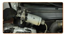
8 Unscrew the water-in-fuel sensor.
