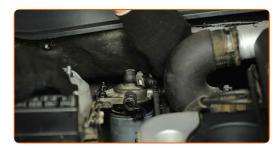
19 Attach the fuel pressure sensor connector.
