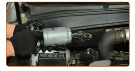
Screw in the water-in-fuel sensor.
