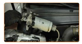
8 Unscrew the water-in-fuel sensor.
