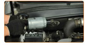
Screw in the water-in-fuel sensor.
